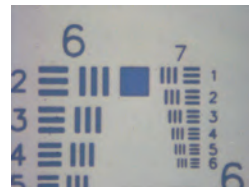
ZRCL-1.5 Observation Field of View About 0.37×0.3mm
