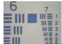
ZRCL-2 Observation Field of View About 0.28×0.22mm
