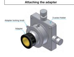
Please connect a fiber connector into the adapter cylinder. 2 Please insert the adapter into the 3-axis holder, and secure it by using the adapter locking knobs located on both ends of the 3-axis holder.
