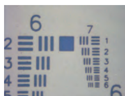
ZRCL-1.5 Observation Field of View About 0.37x0.3mm
